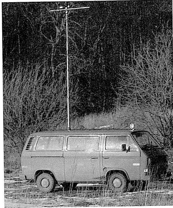
Fig. 2. Bearings of radio-marked red deer were made from a specially equipped mobile unit, a Volkswagen van. The 6-element Yagi-antenna was lifted 6 m above the ground on a pneumatic telescope mast.
