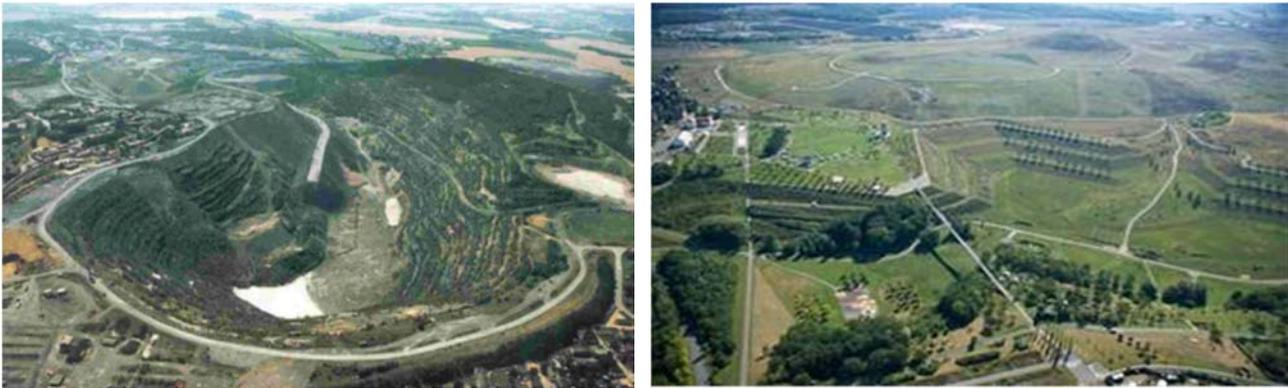
**Figure 8.2.** Backfilling the open pit Lichtenberg in 1992, 2015. Source: <http://www.wismut.de/www/webroot/de/download.php?download=3509>
