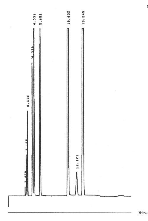
Figur 2: Retentionstider (RT) af standard CFC analyseret som XPS produkter. RT 3,105: CFC 13, RT 3,410: CFC 115, RT 4,239: CFC 1113, RT 4,531: CFC 12, RT 5,652: CFC 114, RT 10,657: CFC 11, RT 13,245: CFC 113.
