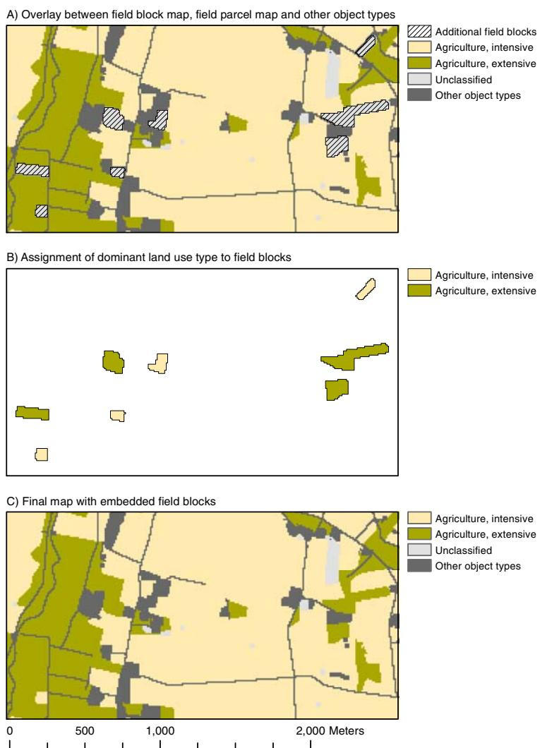
Figure 3.8 Applied method for embedment of field blocks. The field block map, the field parcels map and other types (from LULC00) are overlaid and additional field blocks within yet unclassified areas are selected (A). Based on agricultural registers, the dominant land use type is assigned to each field block (B) and embedded into the final map (C).
