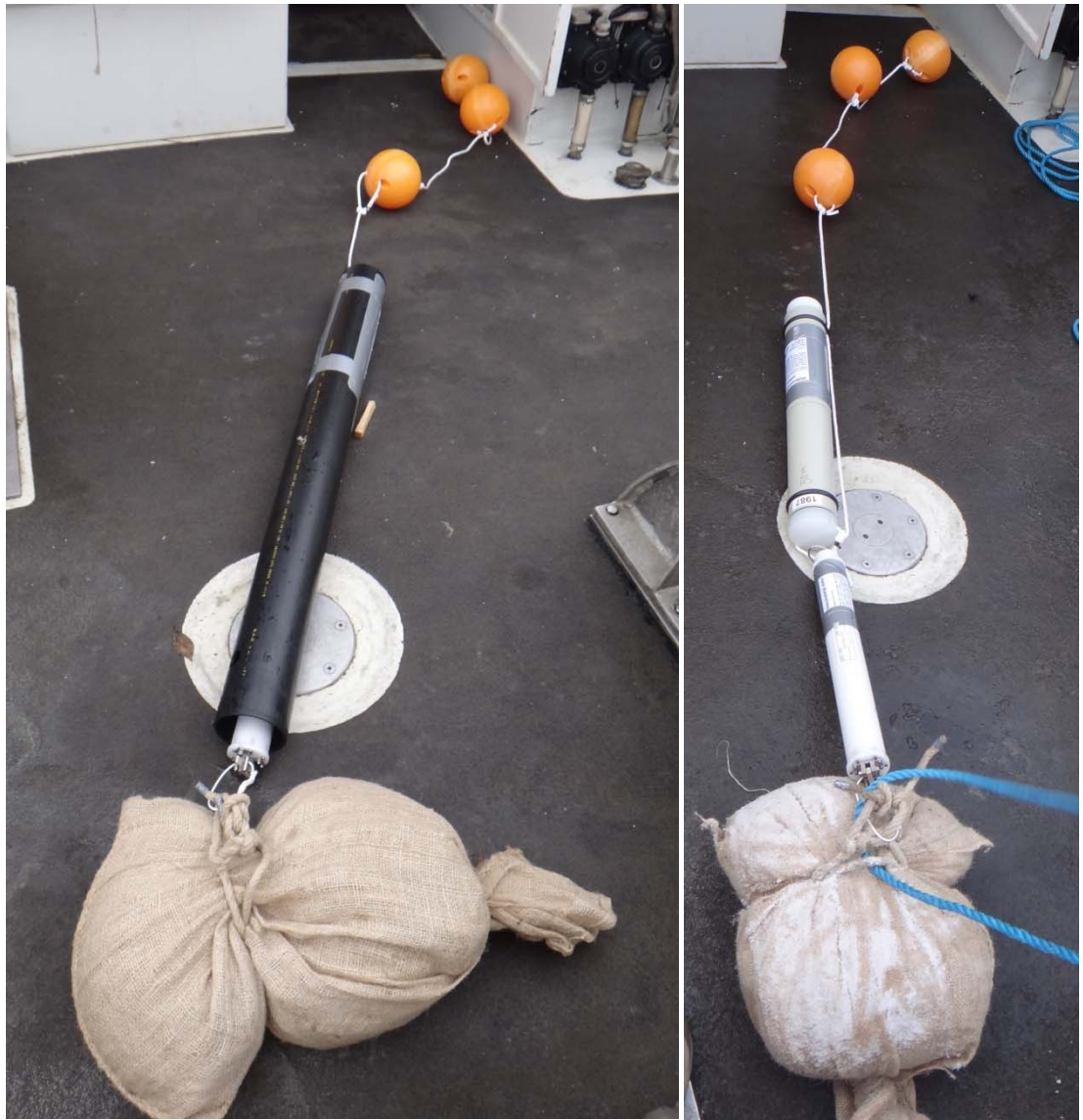
Figure 2.2.1. Acoustic equipment with and without protective tube with the CPOD hydrophone at the top and acoustic release mechanism closest to the sand bags. The orange buoys keep the equipment vertical in the water column and bring the equipment to the surface after release while the sand bags remain at the bottom and are lost.
