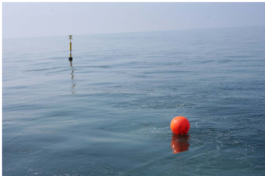
Figure 2.2.3. The buoy system viewed from the surface. The red float is used to retrieve the instruments without pulling the heavy anchor up.
