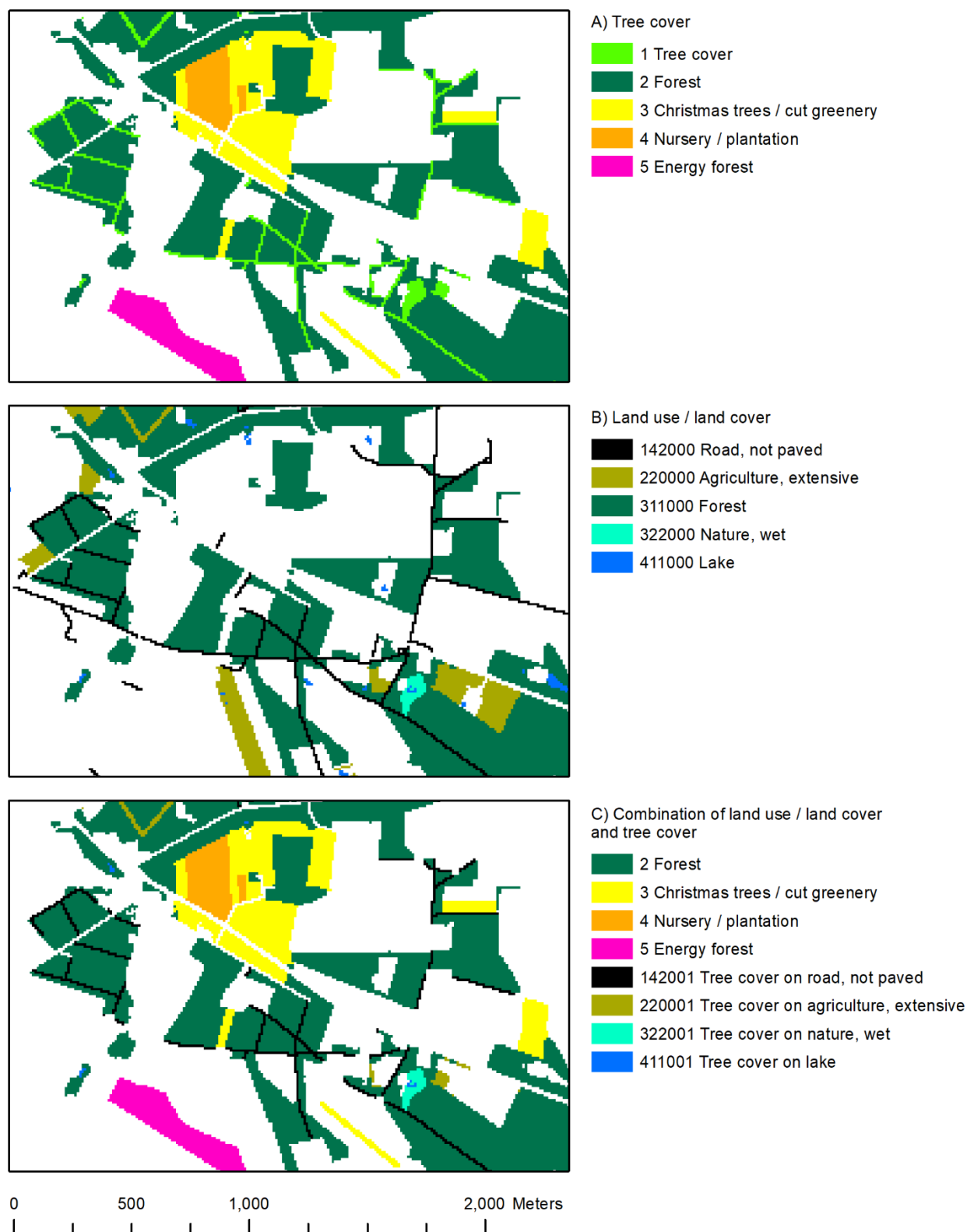
Figure 3.9 Illustration of application of the tree cover layer. From the agricultural census data and the topographical database, areas categorised as tree cover are extracted (A) and overlaid with other land use/land cover categories (B) resulting in different categories of tree cover and combinations of land use/land cover types and tree cover (C)
