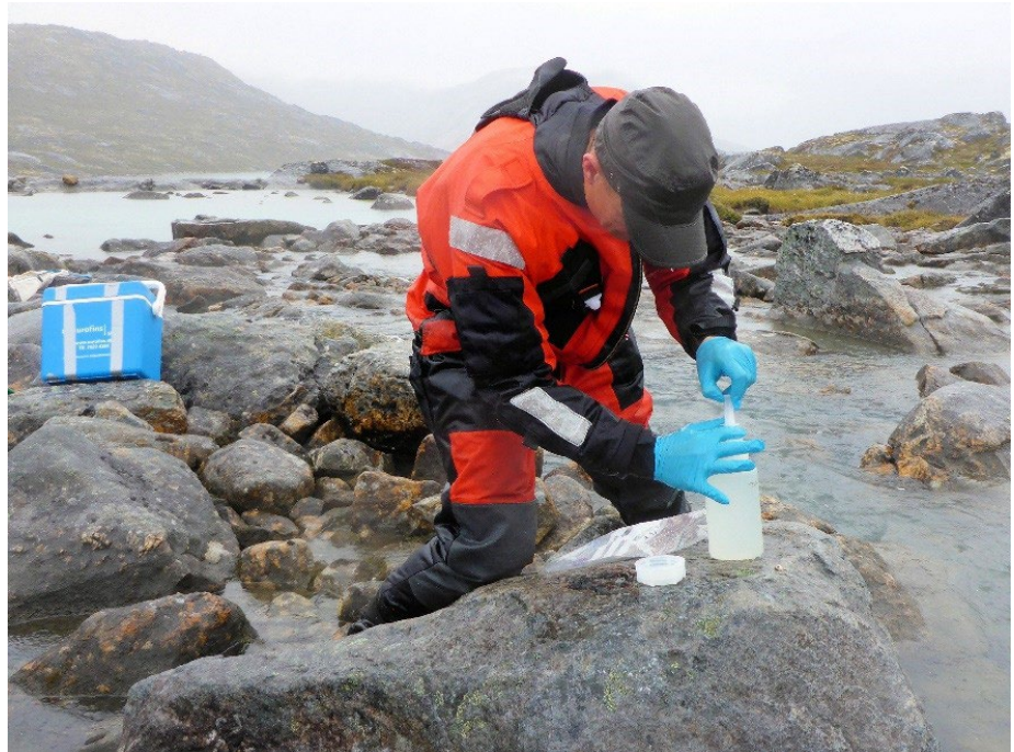
Figure 10. Fresh water sampling. First a clean 1 L bottle is used to take a depth-integrated sample in the stream. Then a syringe is used to take subsamples of unfiltered and filtered water, the latter using disposable 0.45 \mu\text{m} syringe filters, into sample vials. Photo by O. Geertz-Hansen.
