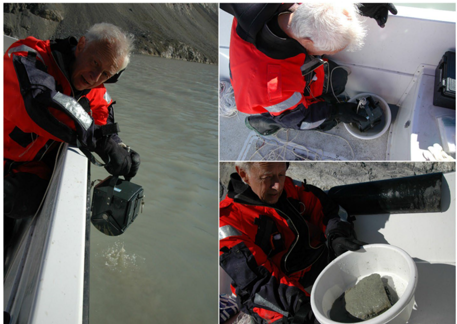
Figure 11. Sediment sampling of bottom surface sediment using an Ekman grab sampler. A slice of bottom surface sediment of 1-3 cm thickness can be obtained. Photos by J. Søndergaard.
