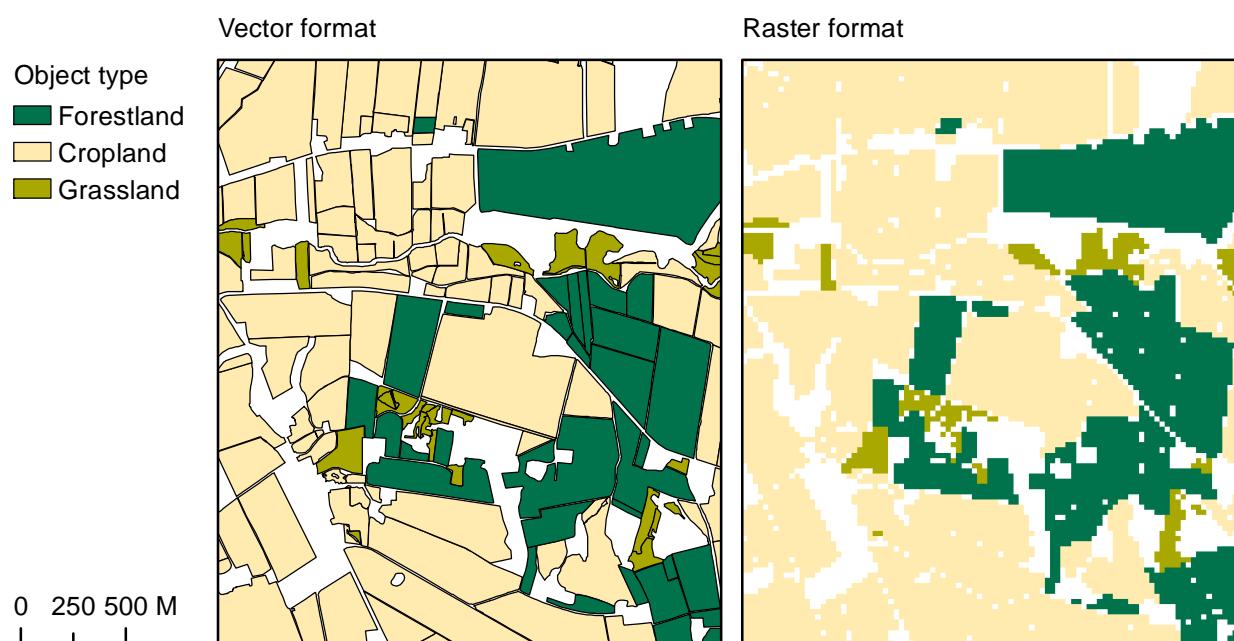
Figure 4.1 Conversion from vector format to raster format illustrated for an extract of the field parcel map.
