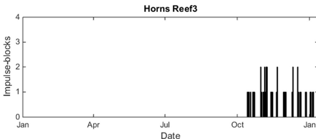
Pile driving of magnitude low (2500 kJ hammer energy), mitigated by means of a bubble curtain (Big Bubble Curtain). Conducted in period from 14.10.2017 to 5.1.2018. In total 49 impulse-block days in 2017, 4 impulse-block days in 2018, distributed over four ICES subrectangles.
