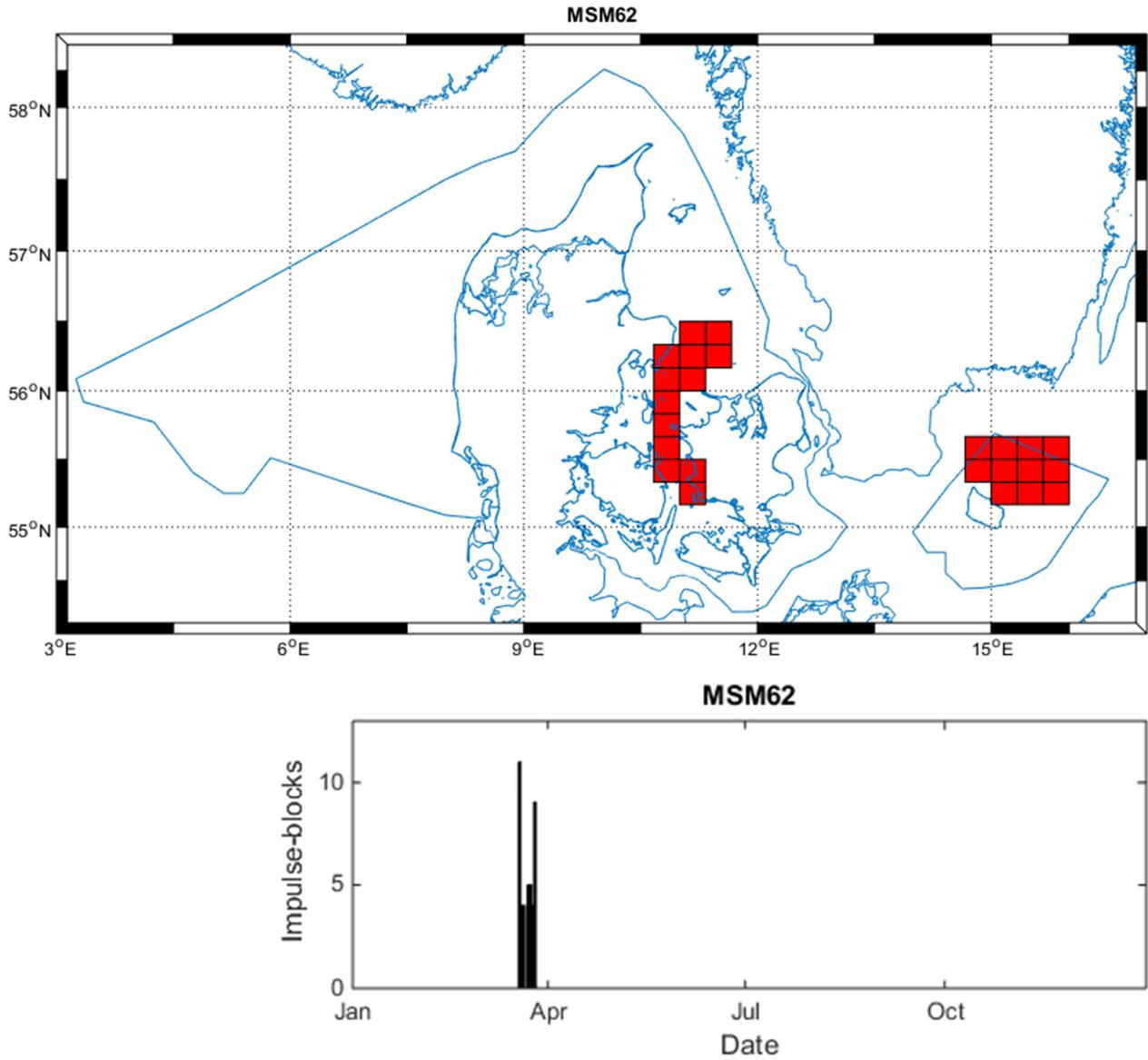
Acoustic survey conducted between 19.3.2017 and 26.3.2017. Type of source not specified further than "Sonar", of magnitude "high". A total of 43 impulse-block days distributed across 24 ICES sub-rectangles.
