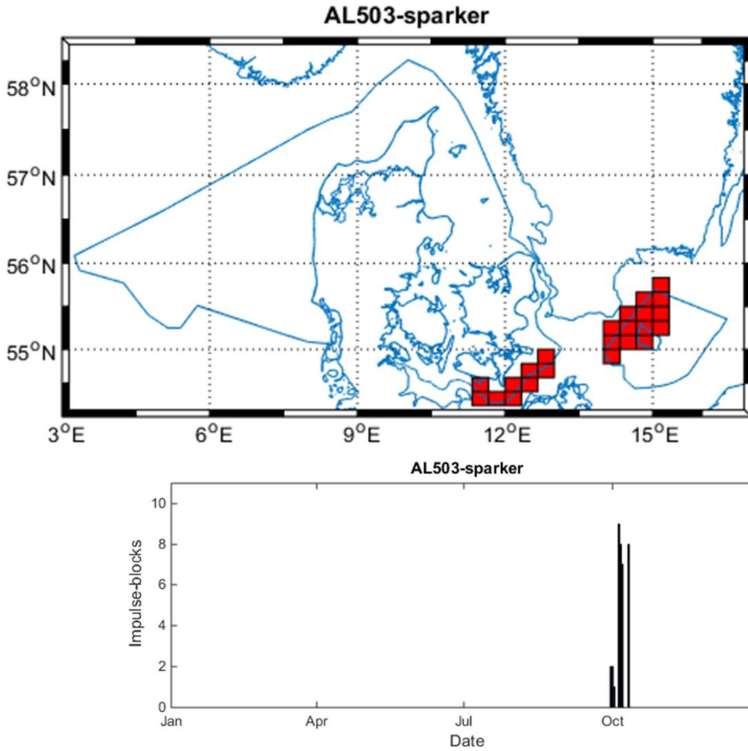
Subbottom profiling with sparker (Innomar SES-2000 medium) of magnitude high. Conducted between 30.9.2017 and 11.10.2017 with a total of 37 impulse-block days.
