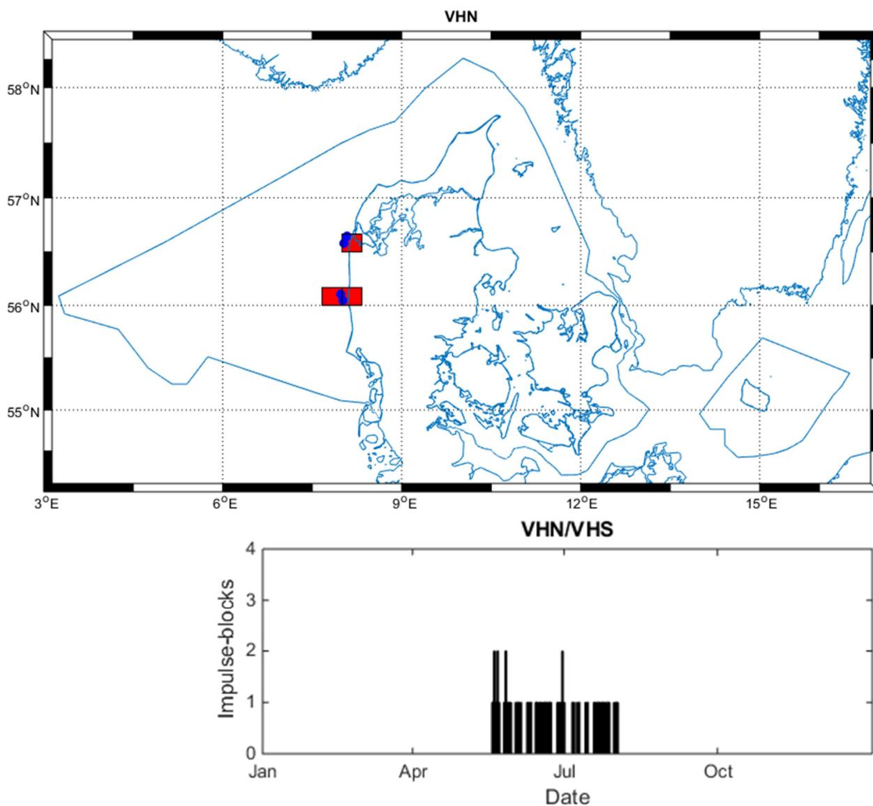
Subbottom profiling with magnitude **very low**. Conducted between 19.5.2017 and 2.8.2017. Source level given as 187 dB re. 1  $\mu\text{Pa}^2\text{s}$ , 221 dB re. 1  $\mu\text{Pa}$  peak. 55 impulse-block days, distributed across three ICES subrectangles.
