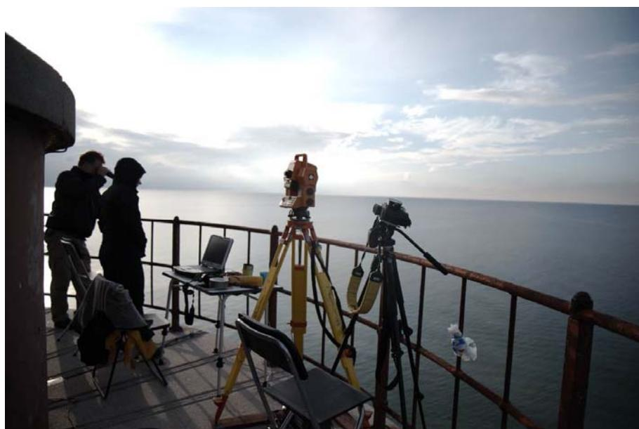
**Figure 2.4.** Setup in the lighthouse with the theodolite (centre), observation stations with binoculars and a small table with a computer connected to the theodolite.
