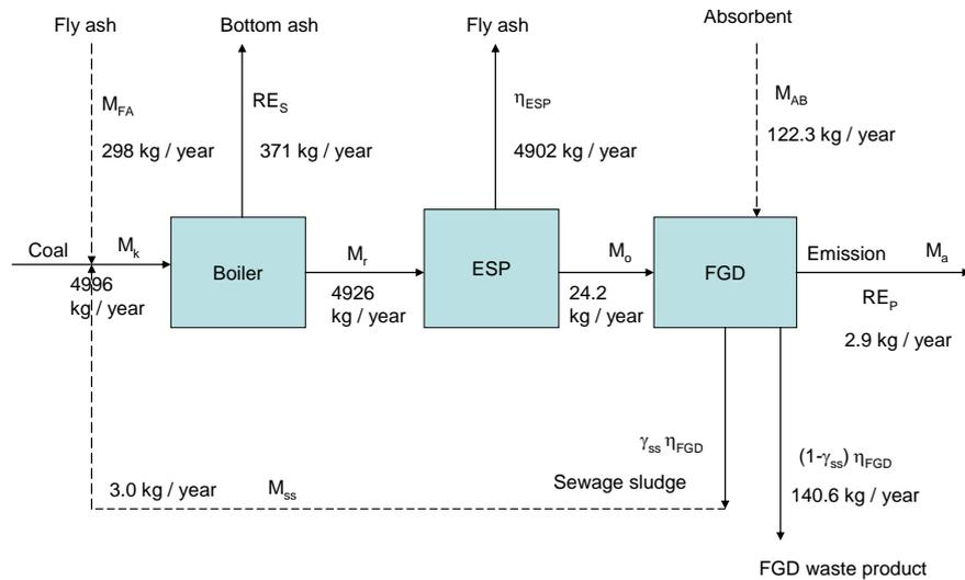
Figure 5.1 The EMOK model for particle bound trace metal emissions, example (Knudsen, 2008).
