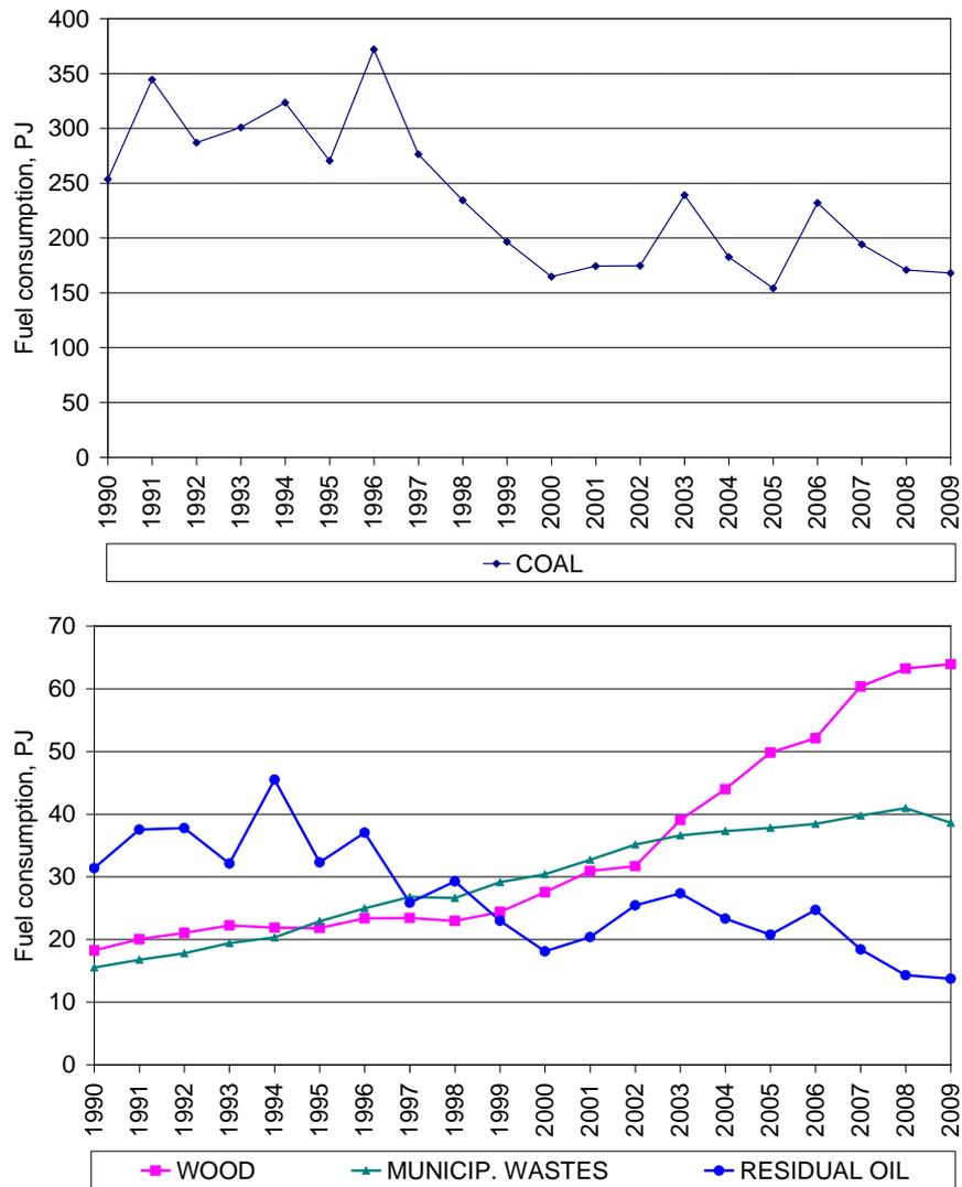
Figure 2.4 Fuel consumption time series for coal, residual oil, waste and wood, stationary combustion. Based on DEA (2010a).
