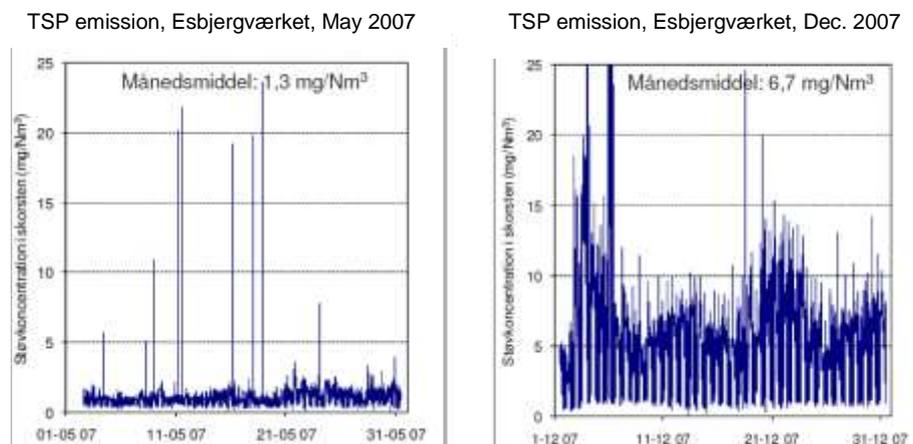
Figure 5.3 Two TSP emission measurements time series for the power plant Esbjergværket (Knudsen 2008).
