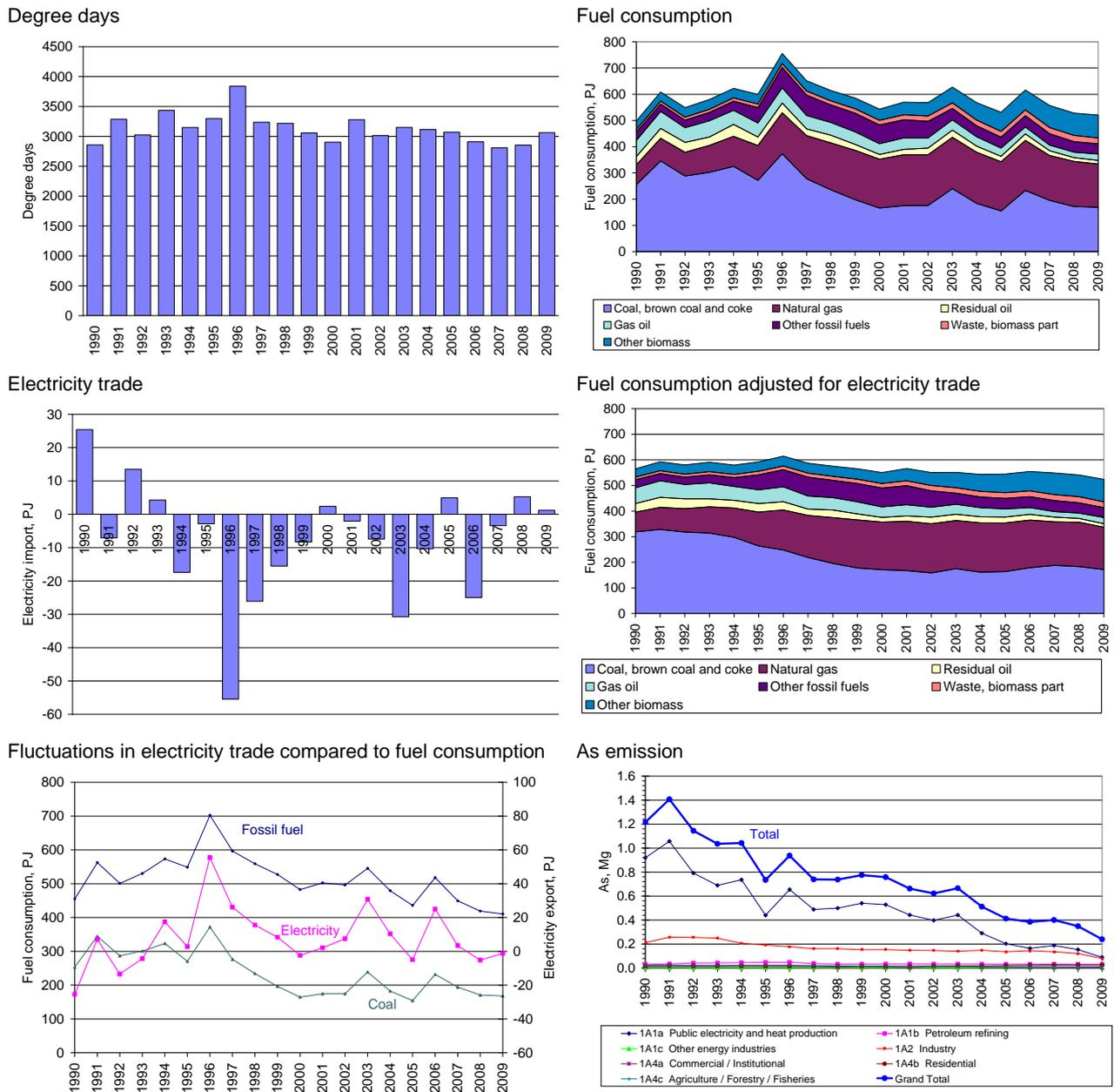
Figure 2.5 Comparison of time series fluctuations for electricity trade, fuel consumption and As emission. Based on DEA (2010a).
