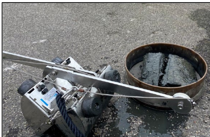
Figure 2.4. Hand-held Van Veen grab and 1 mm sieve used for soft bottom sampling in harbors.
