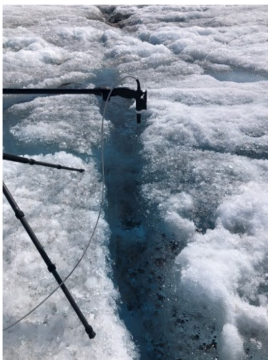
Figure 2.5. The ASD Field-Spec4 during a measurement of field spectroscopy of a cyoconite hole.
