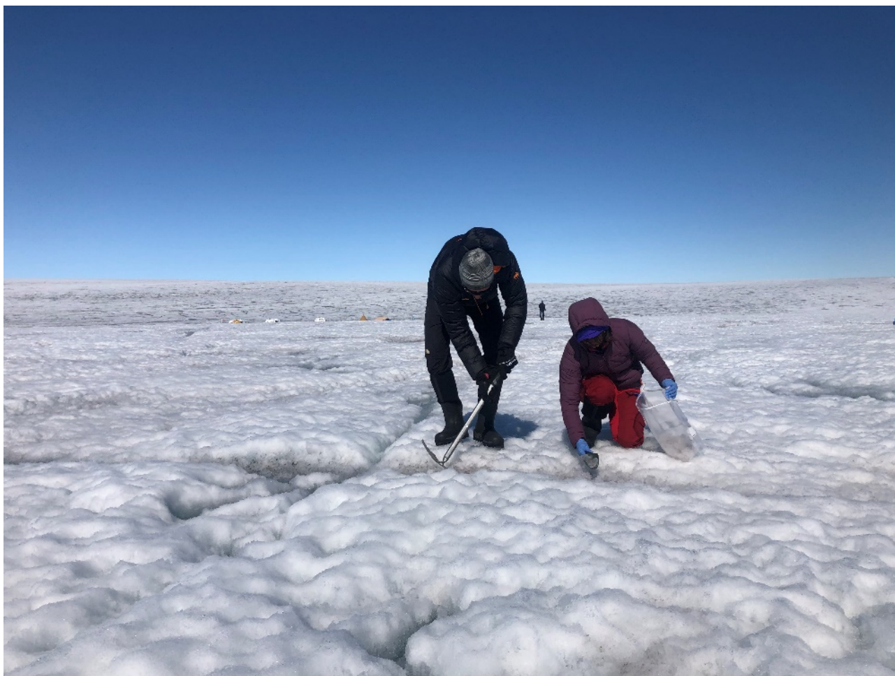
Figure 2.1. Photo of ice scraping procedure using an ice axe. The sampling procedure is ideal for analyses that require large volume of samples, such as DNA, quantification of particulates, elemental analyses, metabolomes (e.g., Lutz et al., 2015, 2016).
