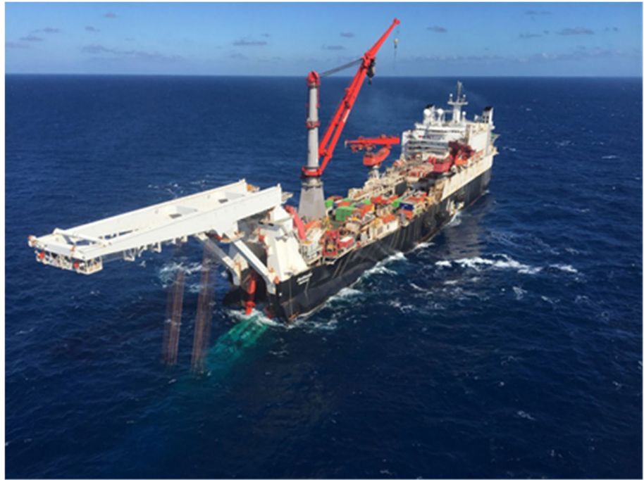
Figure 3.4. Solitaire, the pipe laying vessel used on the Midsjöbanks.
