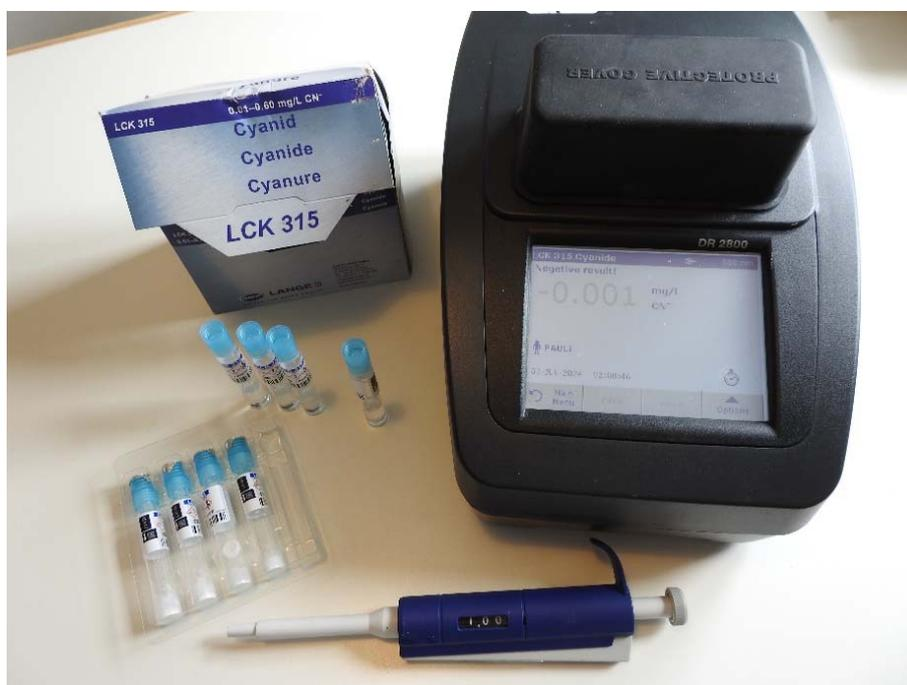
While samples for free cyanide was analysed by the Hach-Lange methods, the samples for total cyanide were sent to an accredited laboratory and analysed for total cyanide by ALS-Denmark after the DS/EN ISO 14403:2002.
