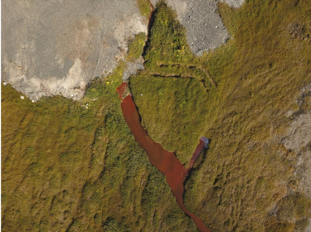
**Figur A10.** Leaching of iron-rich water, which is seen several places at the former camp area.
