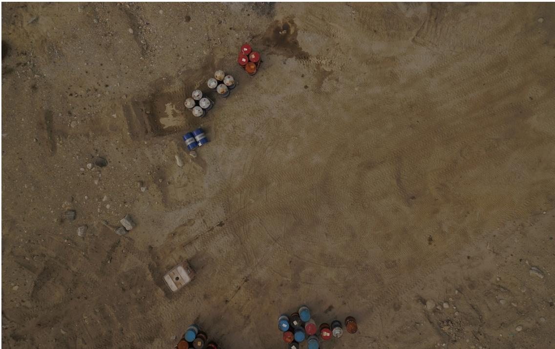
Figure A2-a and -b. Orthophoto from the beach area just west of the new camp, where heavy equipment is landed (a), as well as the actual photo of the area where the fuel barrels are located. At the top of the picture you see staining of the sand around the barrels, which may be due to a spill or possibly rain-water from the top of the barrels.
