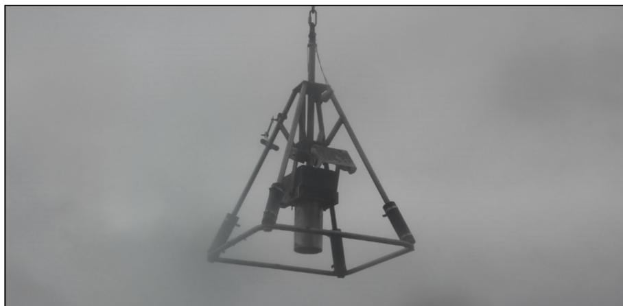
**Figure 4.** Danas' CTD rosette for water sampling and measurements of depth, salinity, temperature, fluorescence, etc.
