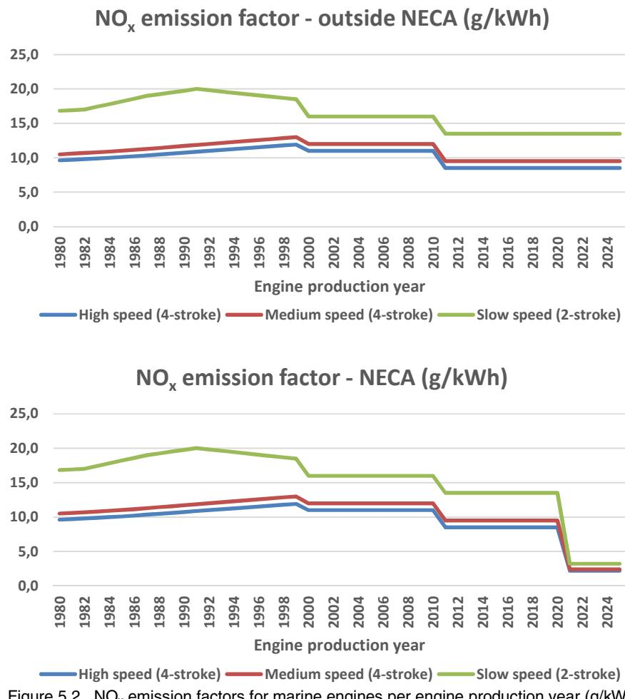
Figure 5.2 NO<sub>x</sub> emission factors for marine engines per engine production year (g/kWh).
