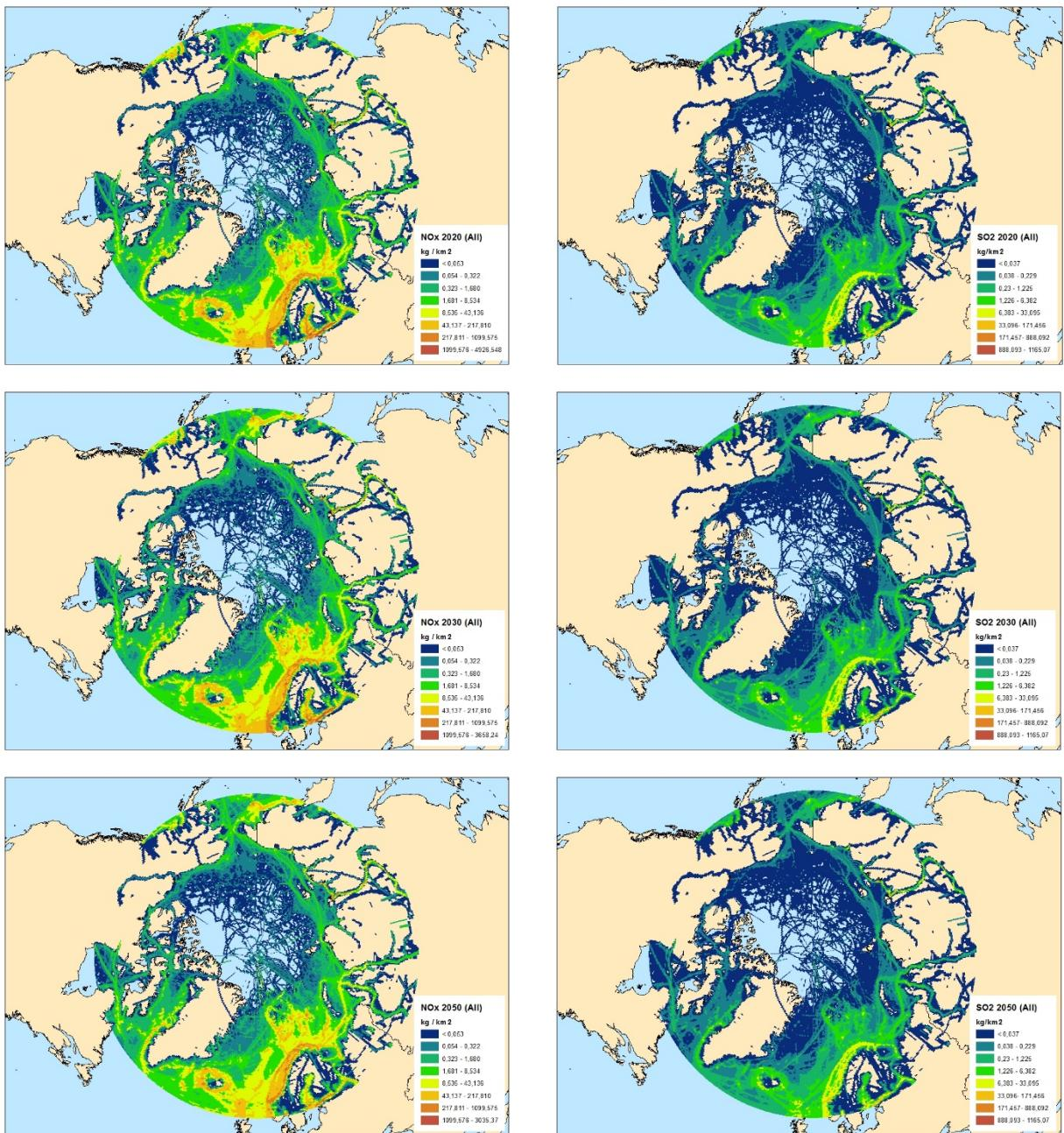
Figure ES 4 Spatial distribution of NO<sub>x</sub> and SO<sub>2</sub> emissions for all ships in 2020, 2030 and 2050 calculated in the Baseline BAU scenario.
