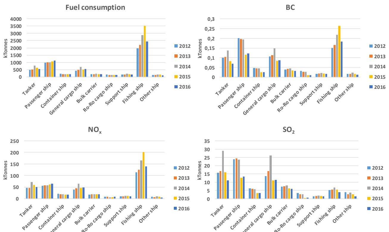
Figure 7.2 Fuel consumption (by mass), NO<sub>x</sub>, SO<sub>2</sub> and BC emissions per ship type in 2012-2016.
