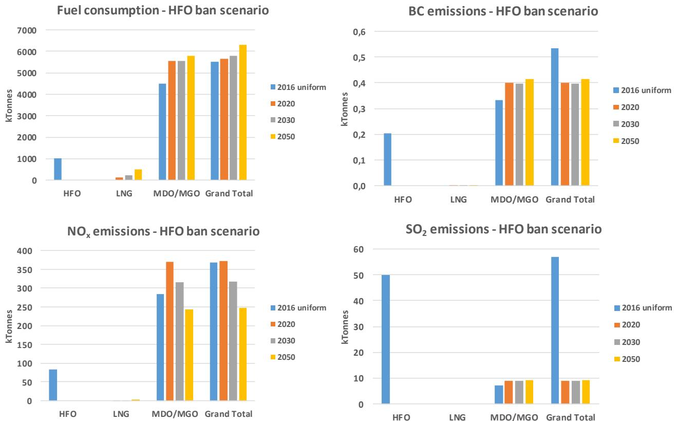
Figure 7.9 Total fuel consumption (by mass), NO<sub>x</sub>, SO<sub>2</sub> and BC emissions calculated in the HFO ban BAU scenario.
