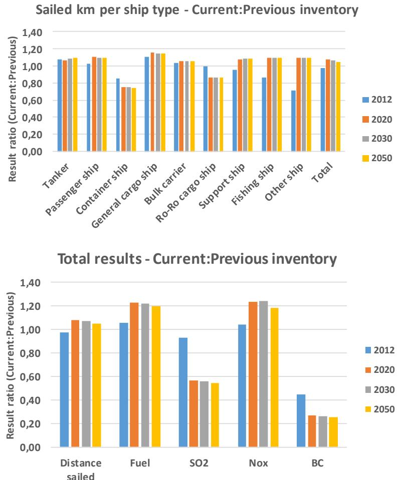
Figure 7.12 Ratios of results for sailed km per ship type (upper figure) and total distance, fuel consumption, SO<sub>2</sub>, NO<sub>x</sub> and BC emissions (lower figure) between current and previous inventory for the years 2012, 2020, 2030 and 2050.
