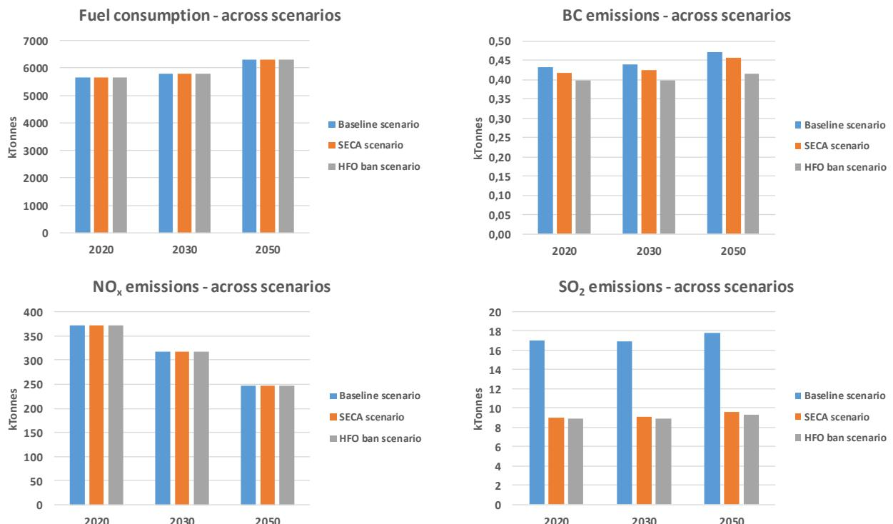
Figure 7.10 Total fuel consumption (by mass), NO<sub>x</sub>, SO<sub>2</sub> and BC emissions calculated in the Baseline, SECA and HFO ban BAU scenarios.
