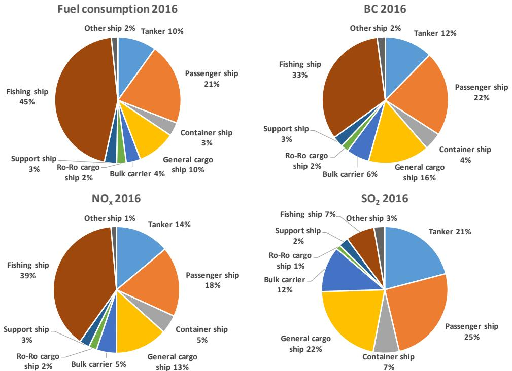
Figure 7.3 Shares of fuel consumption (by mass) and NO<sub>x</sub>, SO<sub>2</sub> and BC emissions per ship type in 2016.
