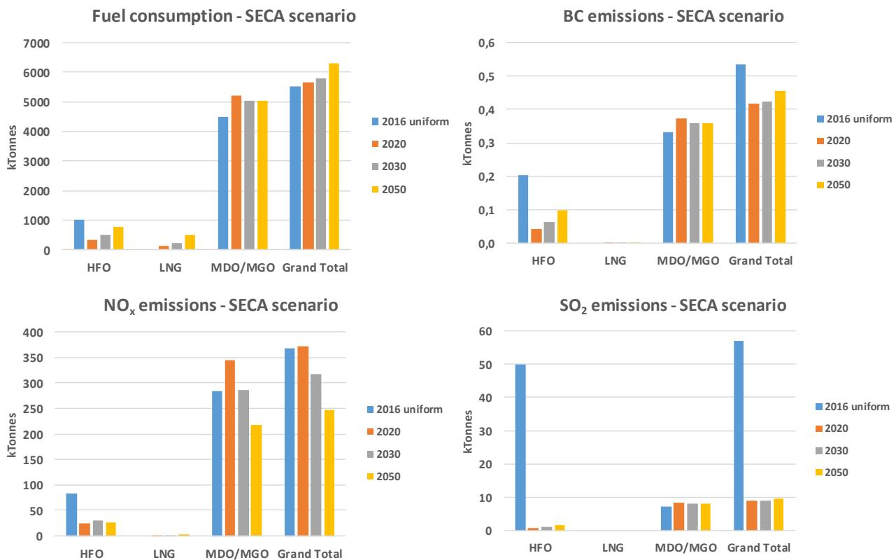
Figure 7.7 Total fuel consumption (by mass), NO<sub>x</sub>, SO<sub>2</sub> and BC emissions calculated in the SECA BAU scenario.
