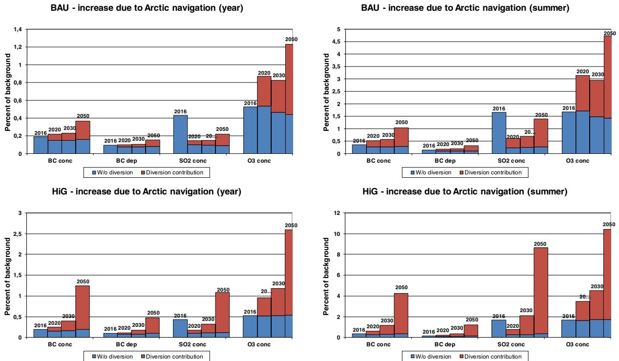
Figure 8.1 Increase of BC deposition and BC, SO<sub>2</sub> and O<sub>3</sub> surface concentrations in 2016 (uniform gridded), 2020, 2030 and 2050 (whole year and summertime average) due to Arctic navigation, as percentage of background.
