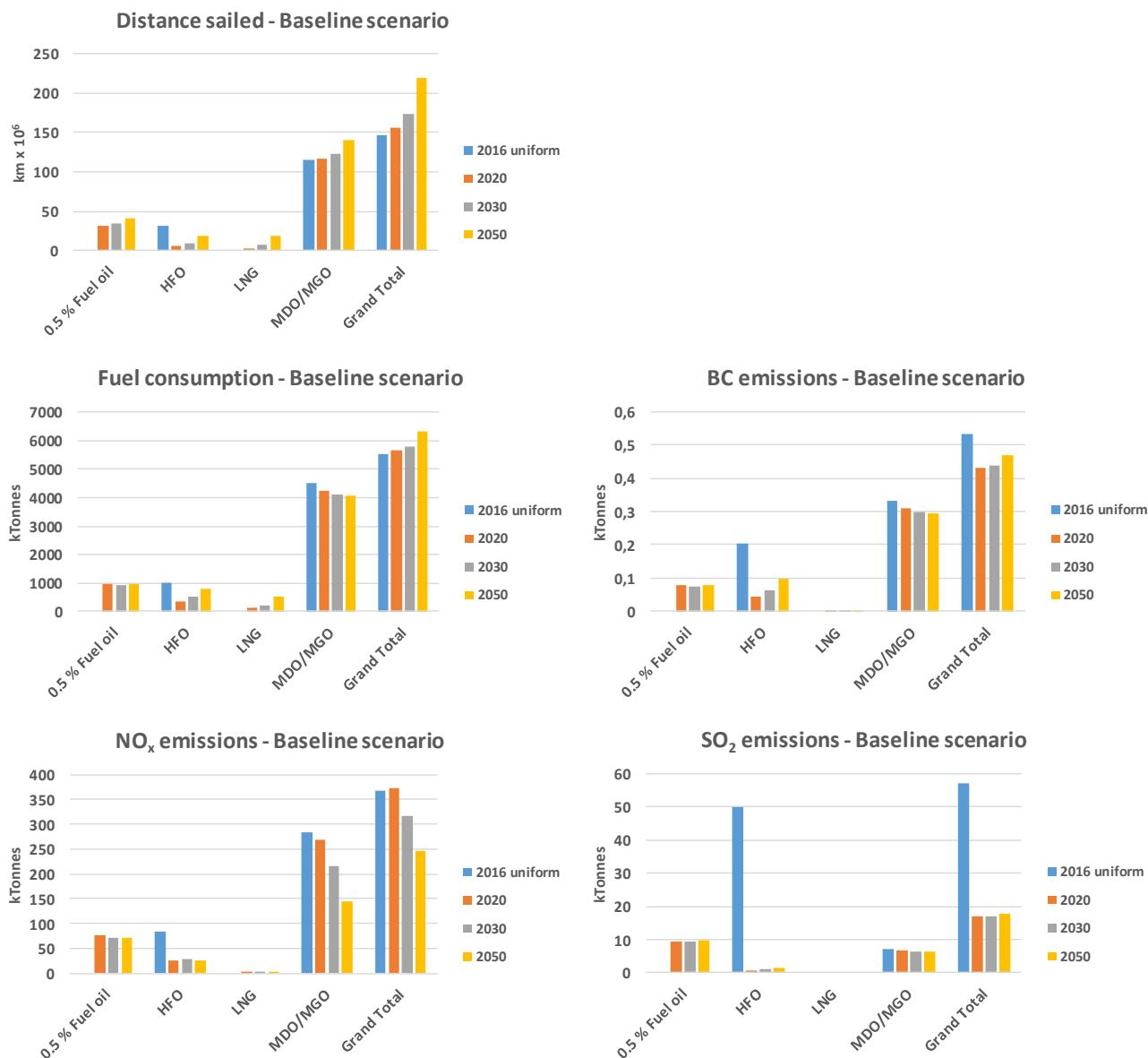
Figure 7.5 Total fuel consumption (by mass), NO<sub>x</sub>, SO<sub>2</sub> and BC emissions calculated in the Baseline BAU scenario.
