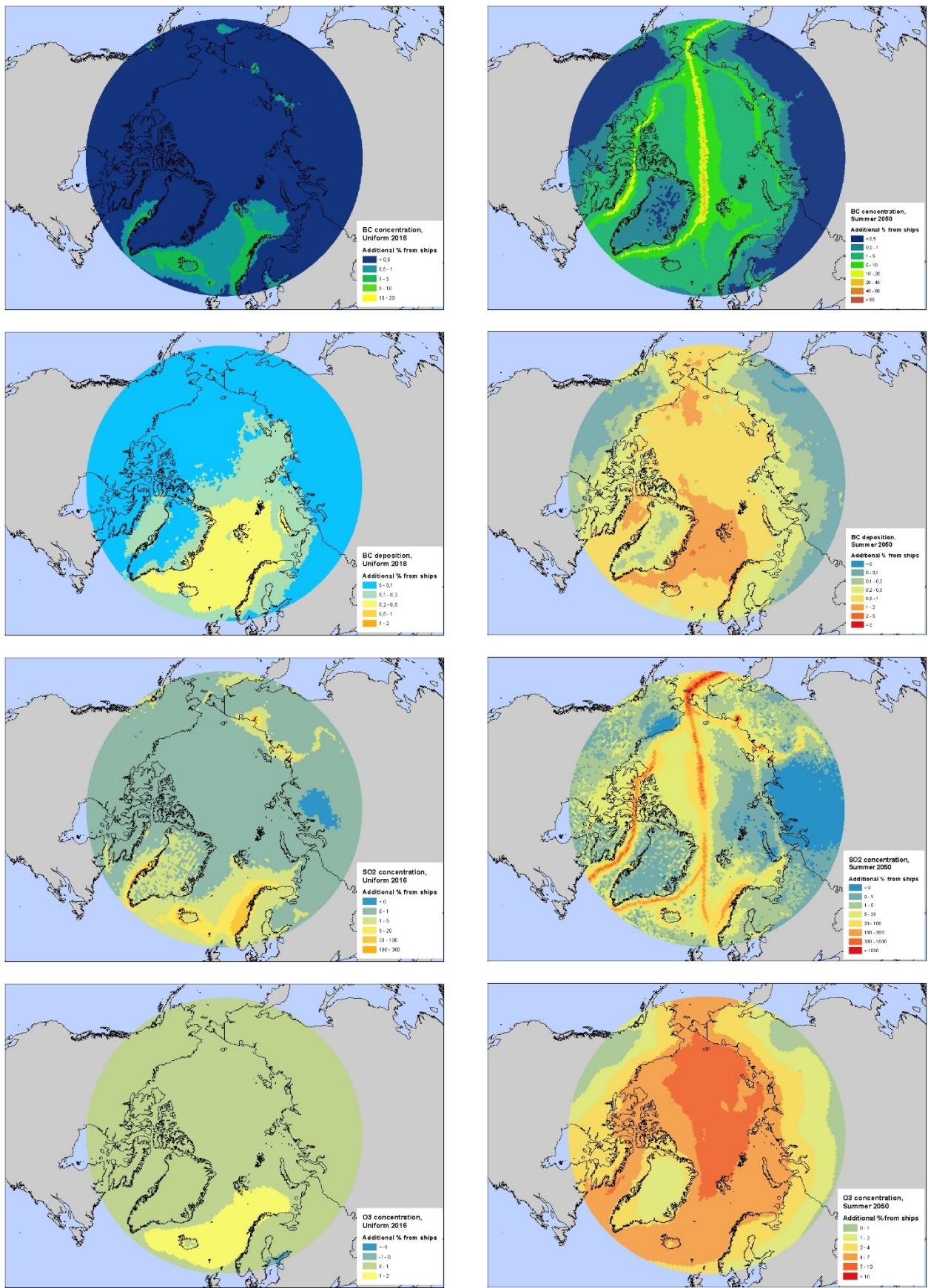
Figure ES 7 Spatial distribution of the increase of BC deposition and BC, SO<sub>2</sub> and O<sub>3</sub> surface concentrations in 2016 (uniform gridded, whole year) and 2050 (summertime) due to Arctic navigation, as percentage of background.
