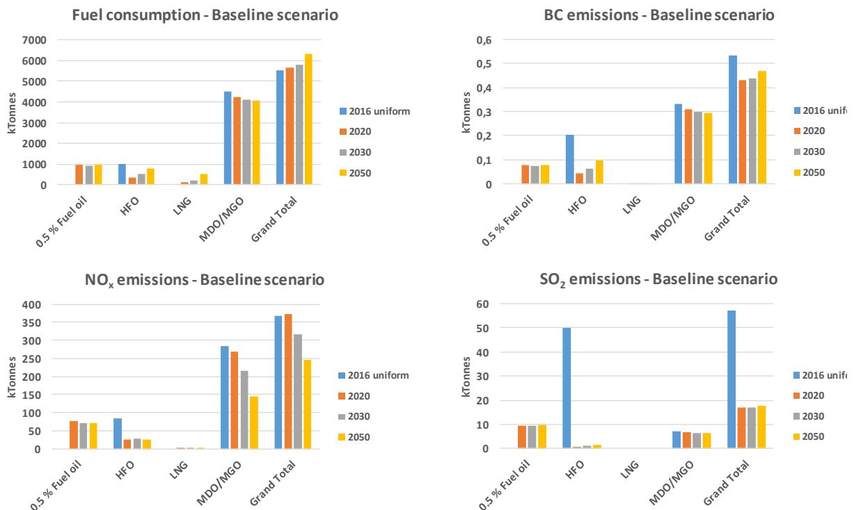
Figure ES 3 Total fuel consumption (by mass), NO<sub>x</sub>, SO<sub>2</sub> and BC emissions calculated for 2016 (uniform gridded) and 2020, 2030 and 2050 in the Baseline BAU scenario.
