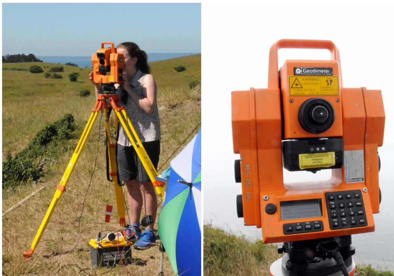
**Figure 2.5.** Theodolite (Geodimeter system 500). Left: setup on tripod and 12V battery. Right: display and keyboard for setup and operation. Adjustment of the theodolite by means of the black dials on the sides. Main sighting scope in the centre of the instrument, auxiliary view finder seen on underside of the black battery box.
