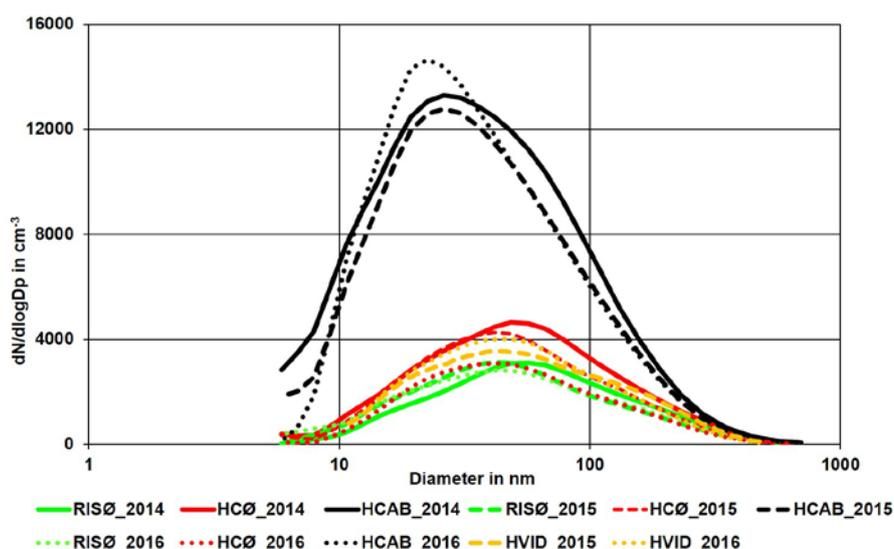
**Figure 2.5.** Yearly averaged particle number size distributions at regional background station RISØ, semi-urban background station HVID, urban background station HCØ and urban curbside station HCAB in 2014, 2015 and 2016.
