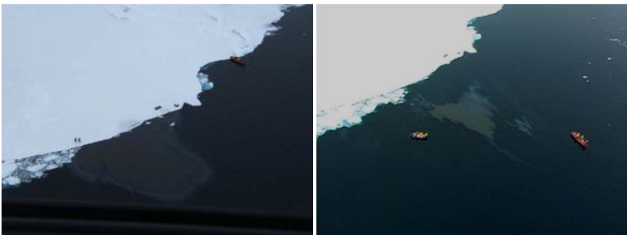
Figure 1.6. Test with herders. Field experiment in the Barents Sea. Left: prior to application of herder, max oil area. Right: area after herder application but before ignition (from SL Ross and DCE 2015).
