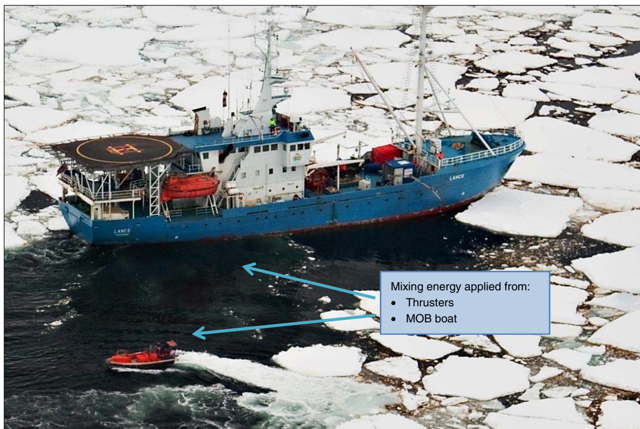
Figure 1.4. Example of an application system of chemical dispersants from a vessel including the use of a rescue boat to create necessary mixing energy (adapted from SINTEF 2013).
