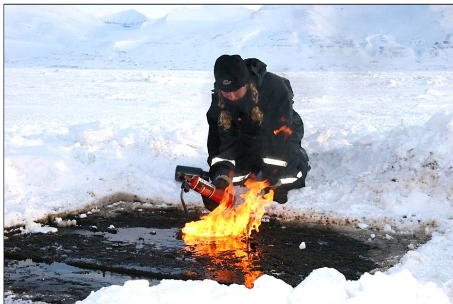
Figure 1.7. Example of a hand-held ignition of an oil slick (from SINTEF 2013).
