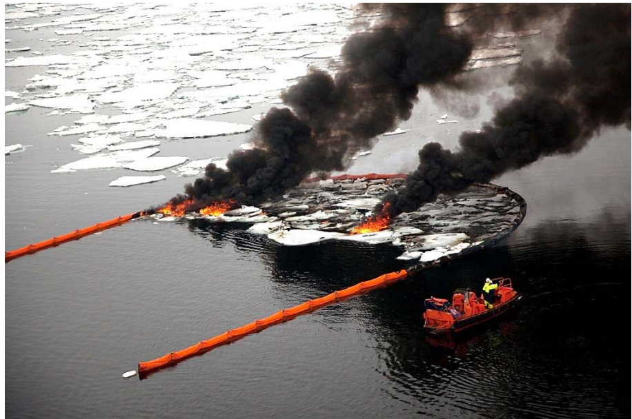
Figure 1.5. Example of an experimental in situ burning operation in the Barents Sea, 2009 (From SINTEF 2013).
