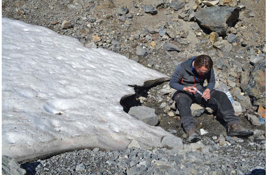
Photo 2.2. Water samples were taken in the water flowing from the mine at the 300 m portal for analyses of cyanide and elements (photo L. Bach).
