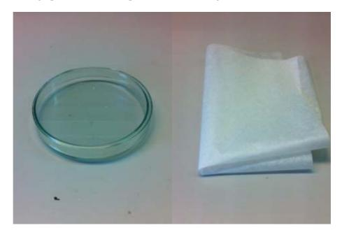
**Figure 19.** Petri dish with a layer of silicone (left) and folded silicone-coated paper (right).
