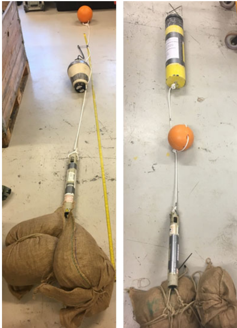
Figure 2.2. Examples of our noise monitoring moorings for the ST500 (left) and SM2M (right). The acoustic releaser is attached to the gravel bags and the recorder attached to the releaser. The orange float provides additional buoyancy to assure that the units reach the surface upon release.
