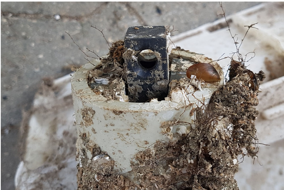
Plastic nut on acoustic release.
