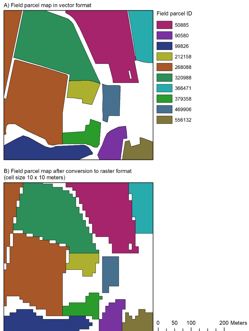
Figure 3.2 Conversion from vector to raster format, exemplified for an extract of the field parcel map.
