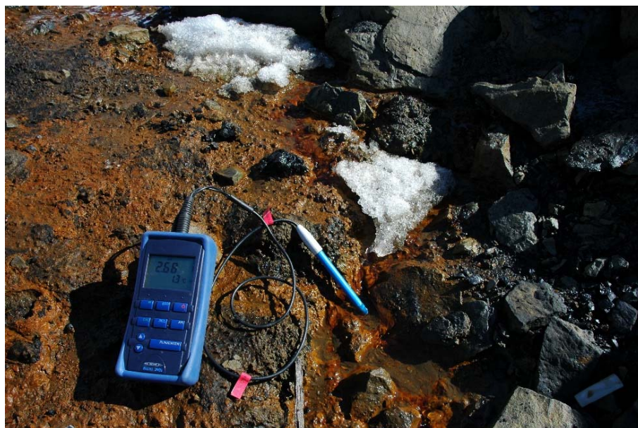
Photo 3. Acid Rock Drainage (ARD) from a coal mine waste rock pile in Svalbard. Precipitated iron hydroxides (also known as ochre) from oxidation of sulphide minerals (mainly pyrite) are visible on the ground surface. Note the pH of 2.68 in the water (Photo: Jens Søndergaard).
